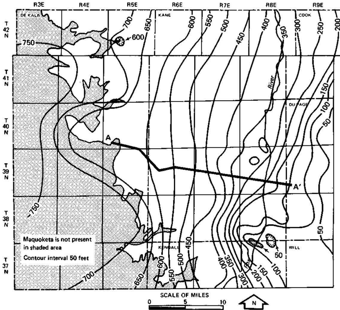
Figure 12. Potentiometric surface of the "Cambrian-Ordovician" aquifer (After Sasman et al., 1986)
