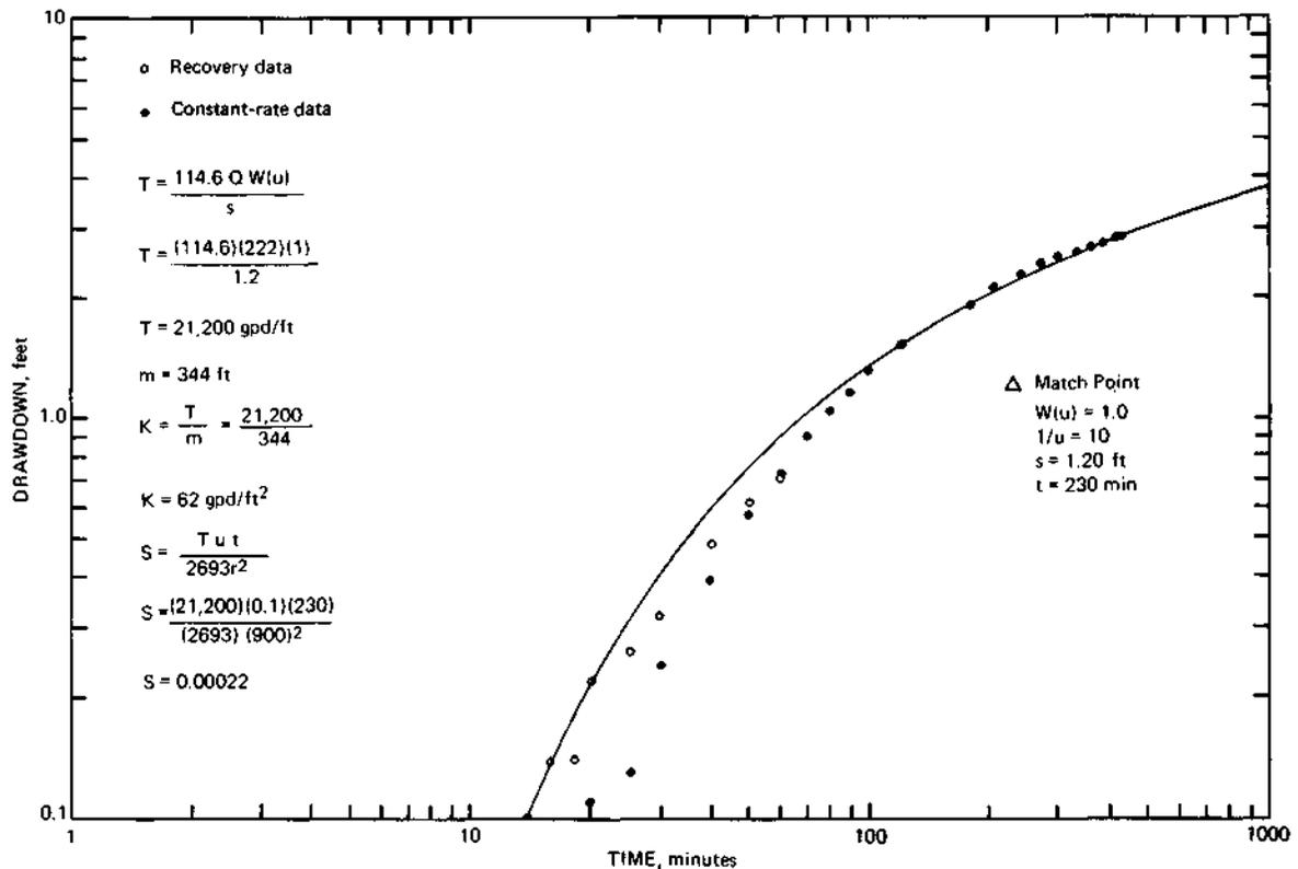
Figure 30. Graphical analysis of time-drawdown data for observation well during Kaneland test
