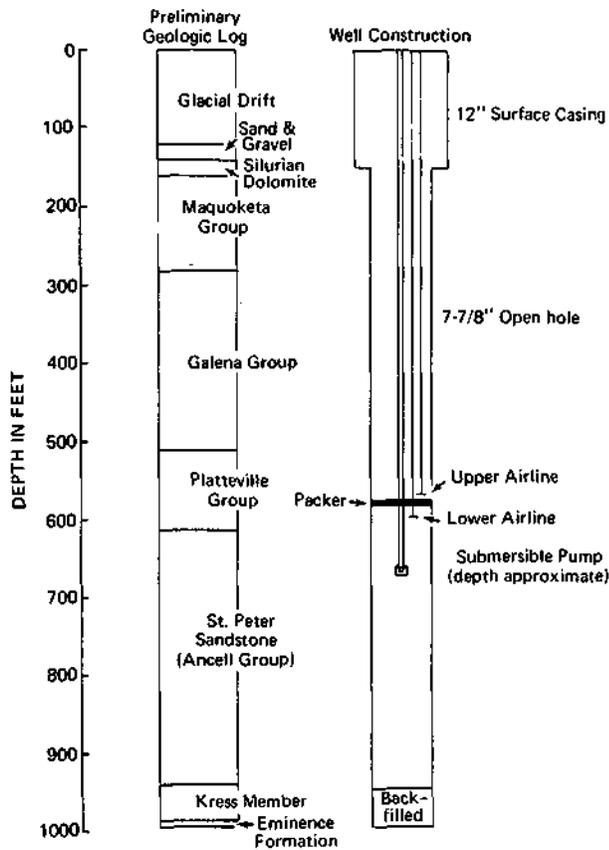
a. Geologic log and construction details for SSC-1
